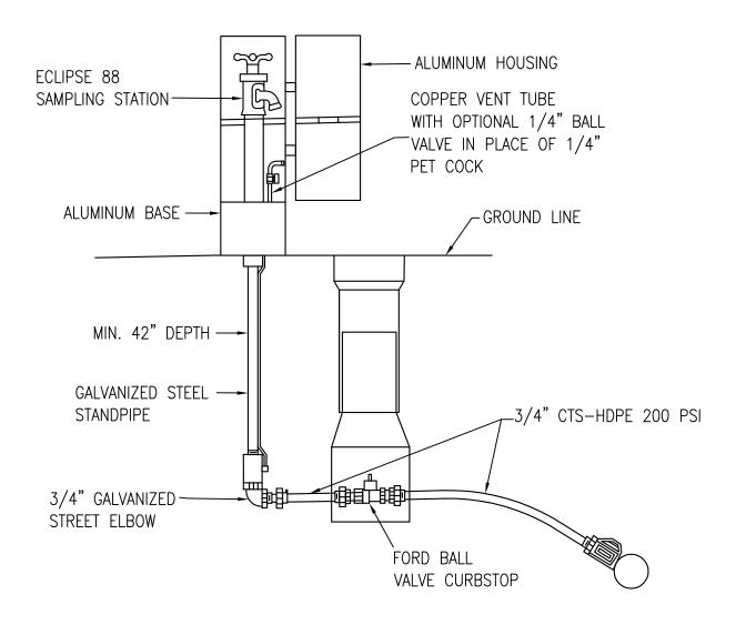
NOTES: THRUST BLOCK DETAIL MUST BE USED TO ANCHOR THE ELBOW AND STANDPIPE FROM SHIFTING.
